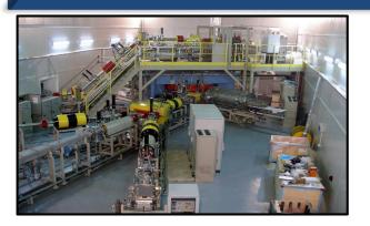
DC-60 -an accelerator of heavy ions for the creation of nano- and micro-structures, modification of materials, research of nuclear reactions.
